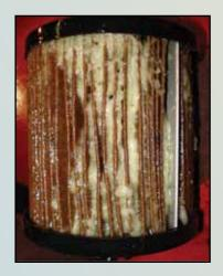
**Paraffin Wax -** Clean filter and hazy fuel. Wax substance in the folds of the filter in temperatures at or below the cloud point.
