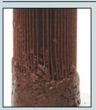
**Sediment -** Granules, sediment in the folds of the filter.
