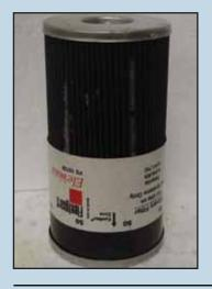
**Microbial Contamination -** Slimy filter with odor, or a black, slimy filter with or without odor.
