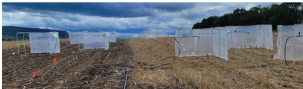
Figure 1. Rainfall simulators used to impose precipitation addition treatments at PSU's research center in Rock Springs, PA.
